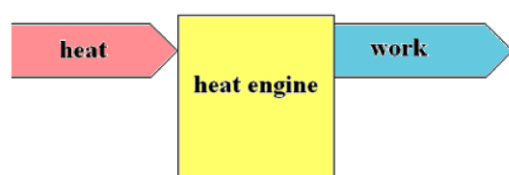
FIGURE 4. A heat engine gets energy as heat and supplies energy as work.
